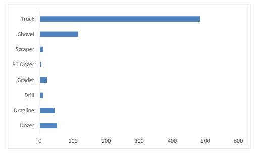
Figure 85: Operational Downtime by Equipment Type – September2019
