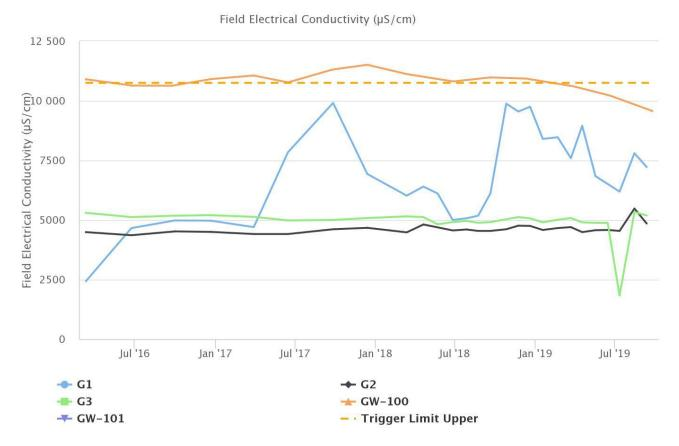
Figure 63: West Pit Alluvium Electrical Conductivity Trend – September 2019
