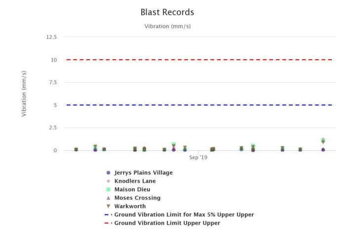
Figure 82: Ground Vibration Blast Monitoring Results – September 2019
